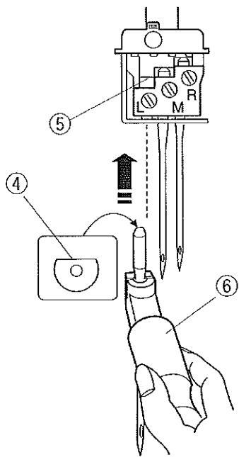
Insert a new needle into the needle clamp with the flat side to the back and push it up against the stopper, then tighten the needle clamp screw.
